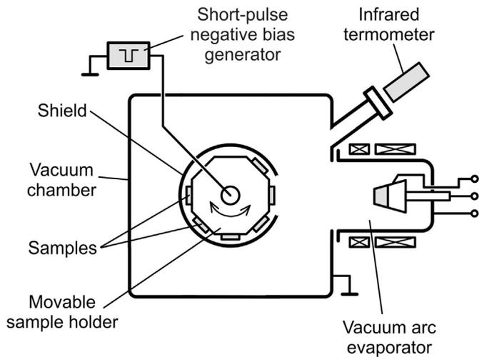
Fig. 1. Scheme of experimental installation.
