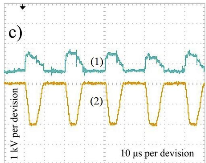
Fig. 2. Oscillograms of negative bias pulses (1) and substrate currents (2) at different frequencies: a –  $1.4 \cdot 10^4$  pps; b –  $2.5 \cdot 10^4$  pps; c –  $5 \cdot 10^4$  pps.
