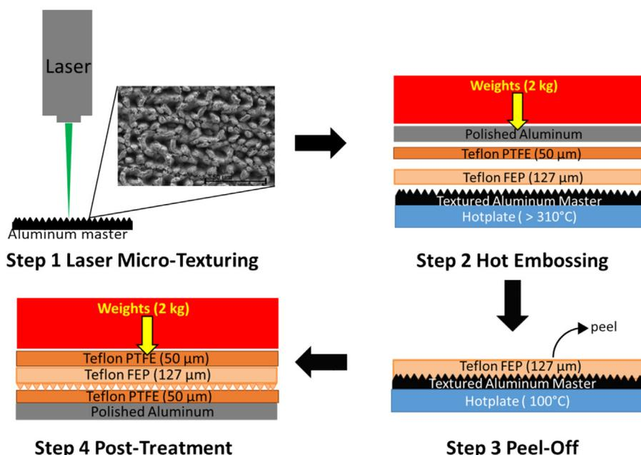
Fig. 1. Schematic showing the four steps required to fabricate a FEP micro-textured superhydrophobic thin sheet.
