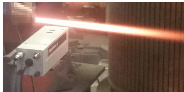
Fig. 1. Spray optimisation using Oseir's SprayWatch system.
