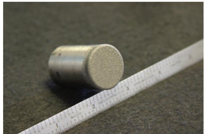
**Fig. 2.** An arc spray coated sample.
