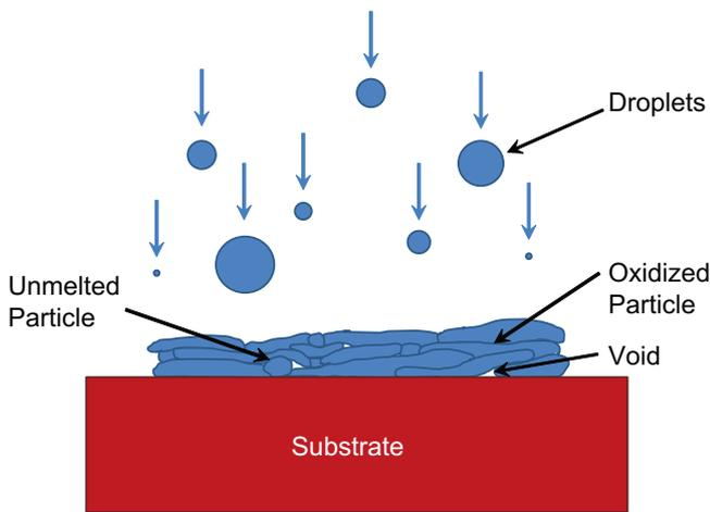
**Fig. 1.** Illustration of the formation of a splat network from thermal spray coating methodologies.
