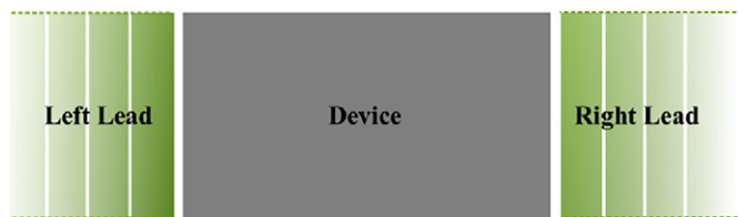
Fig. 1. Schematic view of the system consisting of three parts: left lead, central device, and right lead.
