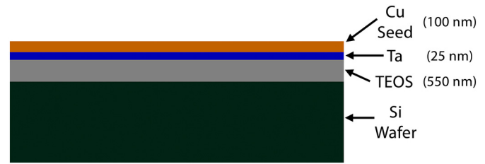
Fig. 1. A cross-sectional illustration of the substrate before copper electroplating.
