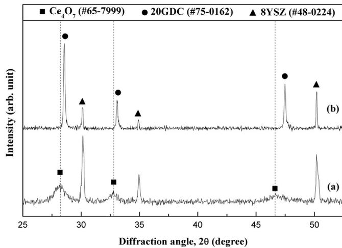
Fig. 1. XRD patterns of (a) as-deposited and (b) 900 °C-annealed 20GDC films on 8YSZt samples.
