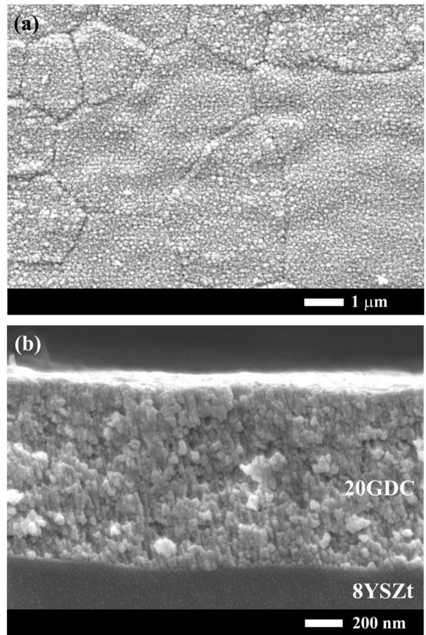
Fig. 3. SEM images of 900 °C-annealed 20GDC/8YSZt samples (a) plane view and (b) cross section.
