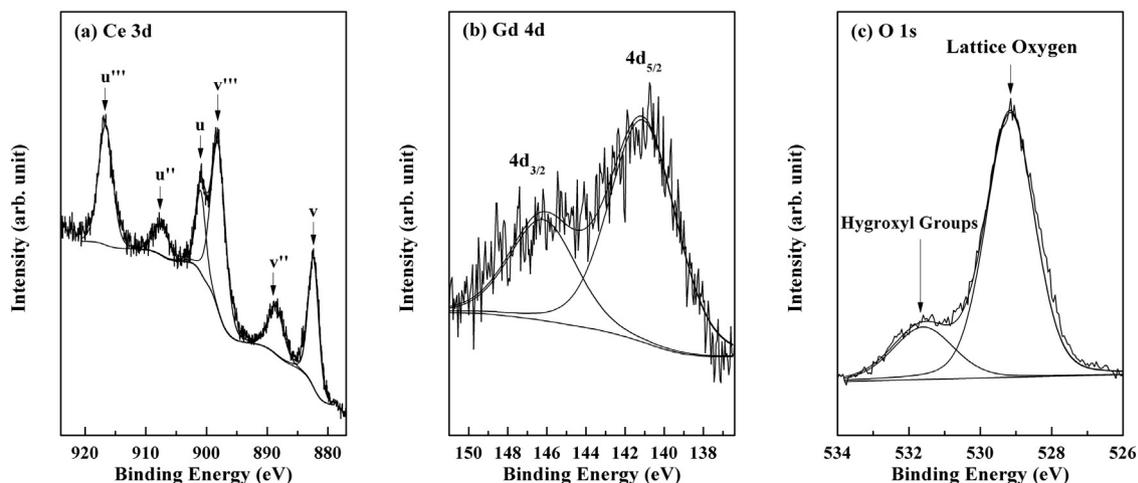
Fig. 2. XPS spectra of (a) Ce 3d, (b) Gd 4d, and (c) O 1s core levels for the 900 °C-annealed 20GDC films on 8YSZt samples.
