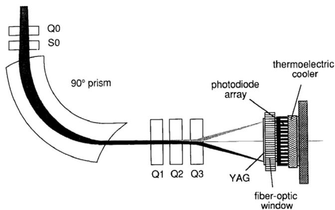
**Fig. 1.** Schematic diagram of Gatan parallel EELS showing the magnetic sector, the pre-sector focusing coils, post-spectrometer lens assembly, and the photodiode detection system. From O.L. Krivanek et al. [12].
