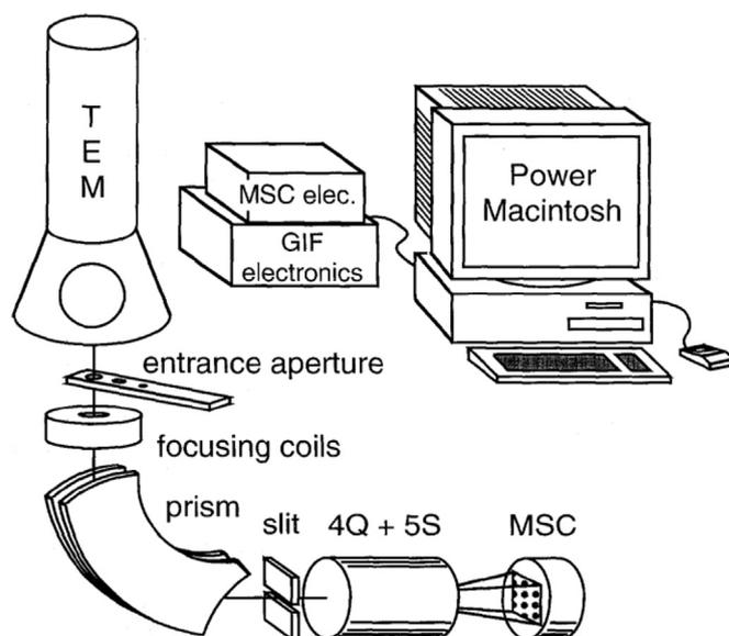
**Fig. 2.** Principal components of the Gatan imaging filter system: (Q) quadrupole lens, (S) sextupole lens, (MSC) multi-scan CCD camera, (GIF) Gatan imaging filter. From O.L. Krivanek et al. [18].
