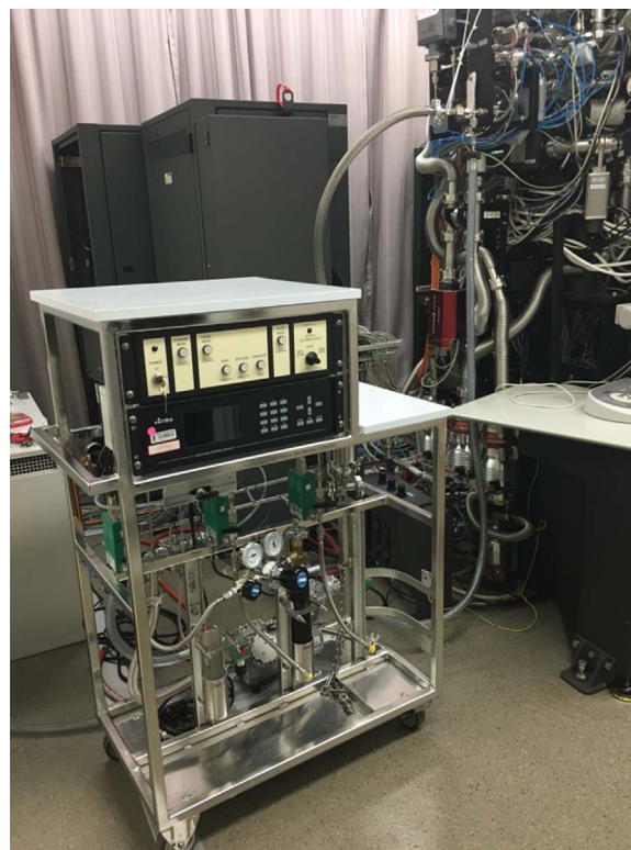
Fig. 1. Photograph of the gas mixing console beside the ETEM.
