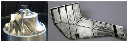
Fig. 2. Examples of machining of titanium impellers.
