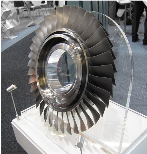
Fig. 1. A compressor blisk on display at the Paris Air Show 2013. This is a single-piece item, generated with 3D CNC milling. Source: Olivier Cleynen; license: CC BY-SA 3.0.
