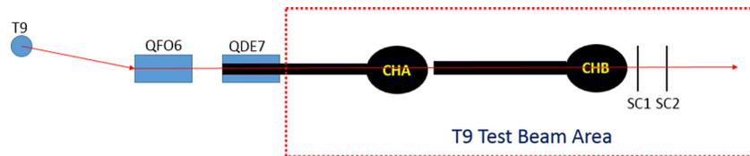
**Fig. 1.** Schematic drawing of the experimental setup in T9. The red arrow corresponds to the beam trajectory, passing through two quadrupoles designated “QF06” and “QDE7” and then traversing the two Cherenkov detectors “A” and “B”, filled with CO<sub>2</sub>. After the Cherenkov detectors two scintillators in coincidence (SC1 and SC2) are placed.
