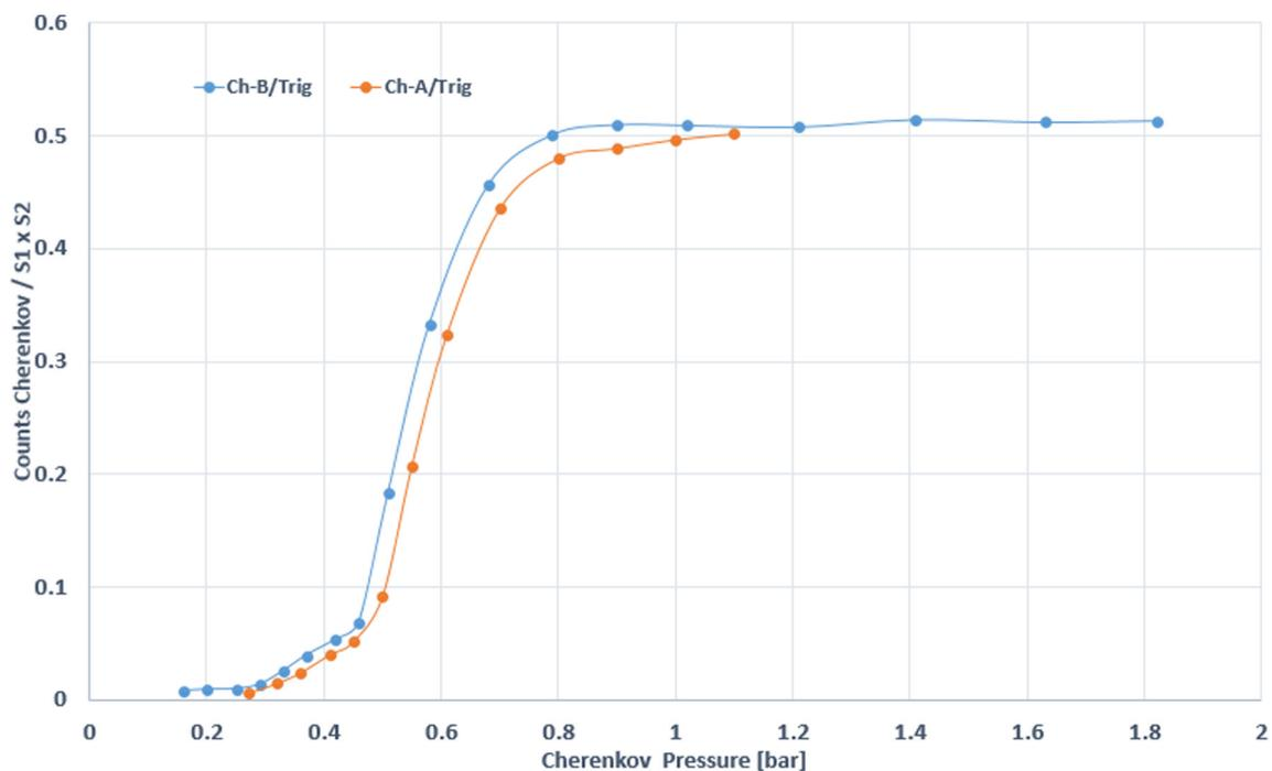
**Fig. 2.** Pressure scan for both Cherenkov A and B detectors, starting from the Cherenkov light threshold pressure for pions. The y-axis is the ratio of the counts of each detector divided by the trigger counts.
