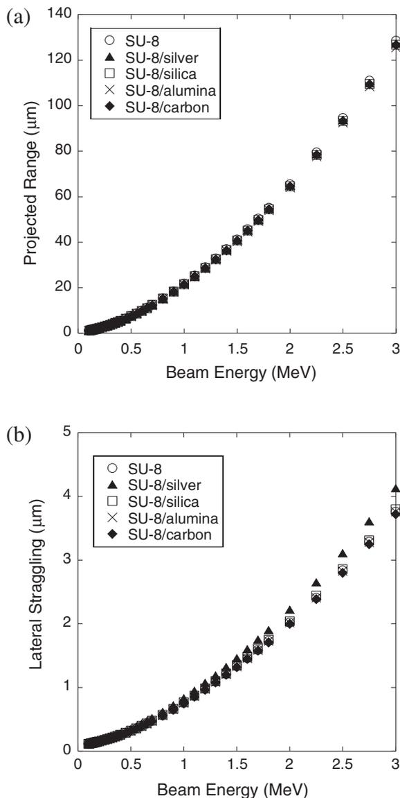
**Fig. 1.** SRIM simulation for SU-8 and SU-8/nanoparticles composites with 5.0 wt% in SU-8. Projected ranges (a) and lateral stragglng (b) in SU-8/nanoparticles composites.
