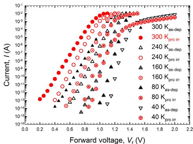
Fig. 1. Semi-logarithmic forward  $I$ - $V$  characteristics of Au/Ni/4H-SiC Schottky diodes before and after proton irradiation at a fluence of  $2.0 \times 10^{12} \text{ cm}^{-2}$ , measured at different temperatures between 40 K and 300 K.
