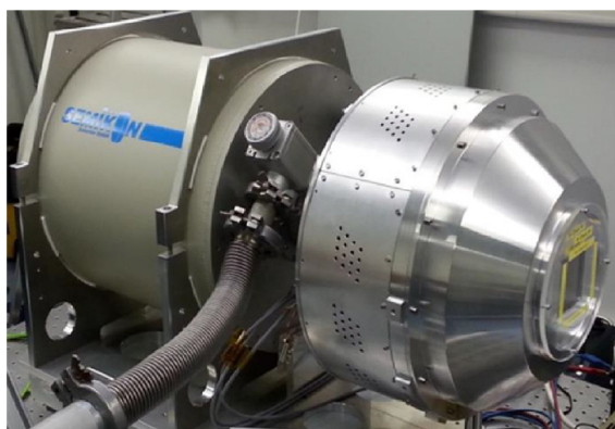
Fig. 1. Left: New Si(Li) polarimeter system including LN 2 Dewar. Right: schematical drawing of the segmented detector crystal (right).
