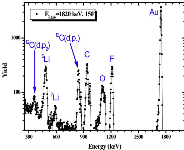
Fig. 1. Experimental deuteron spectrum at  $E_{d,lab} = 1820$  keV and 150°, along with the corresponding peak identification.
