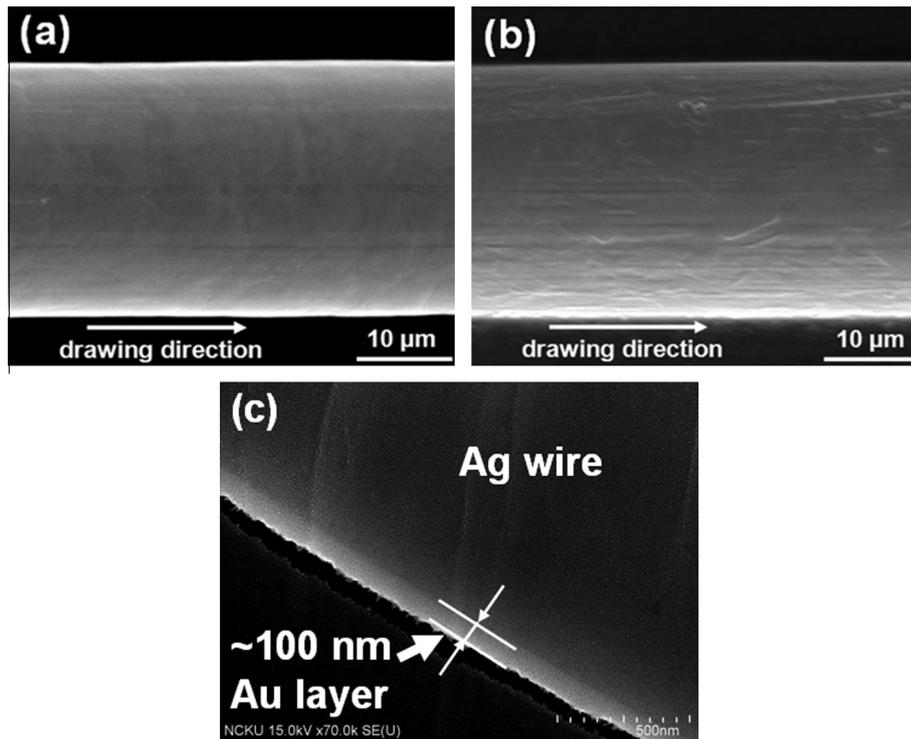
Fig. 2. Surface characterizations of the fine wire. (a) Ag; (b) ACA and (c) cross-section of ACA wire.
