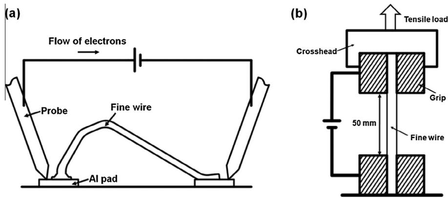
Fig. 1. Schematic diagram of the equipments. (a) Measurement system for fusing current test of fine wire; (b) mechanism for tensile test on wire in current loading.
