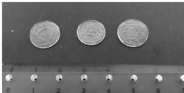
Fig. 1. The photograph of the fabricated Dy 3+ -doped CaO–Al 2 O 3 –B 2 O 3 -based glass samples. From left to right, Dy 3+ concentration is 0.5, 1.0, and 2.0 mol%.
