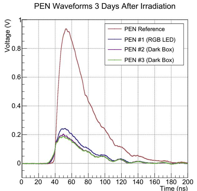
Fig. 2. PEN average waveforms three days after 100 kGy irradiation.
