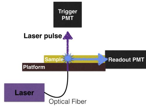
Fig. 1. Sketch of the setup used to measure the scintillation performance of the tested scintillators.
