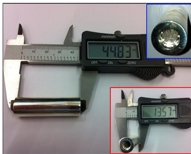
Fig. 2. Cylindrical PSL manufactured using 3D printing.
