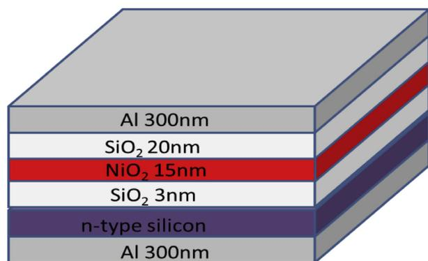
Fig. 1. NiO<sub>2</sub> flash memory device structure.
