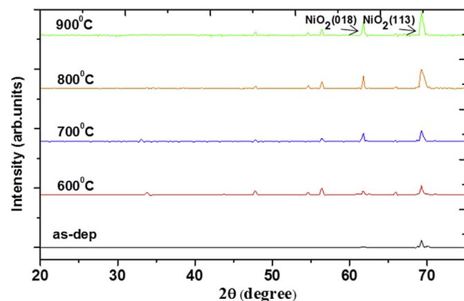
Fig. 2. XRD of the as-deposited film and the films after RTA annealing treatment at 600 °C, 700 °C, 800 °C, and 900 °C.
