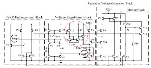
Fig. 2. Schematic of the proposed BGR.
