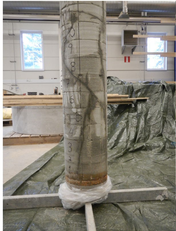
Fig. 1. Example photograph of the Hole 18 bentonite parcel. The bentonite parcel height visible in the picture is about 1 m. The thin horizontal circular rings are the limits between different numbered compacted bentonite blocks (each of about 10 cm height except block 2). The thin vertical black line is the 0° reference line with increasing angles clockwise in the figure. Other dark patterns are believed to correspond to rock fracture traces (credits: Mattias Åkesson and Clay Technology).
