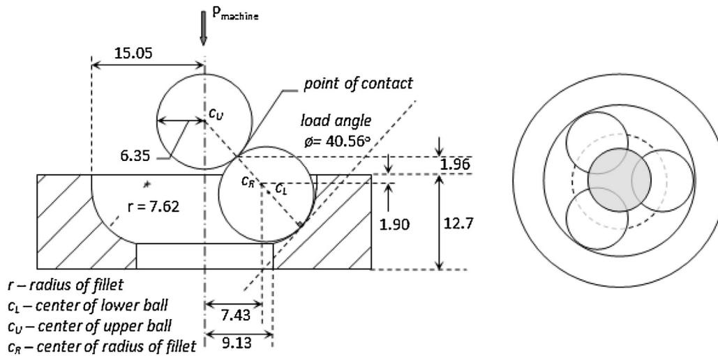
Fig. 1. Ball configuration in the four-ball tester.
