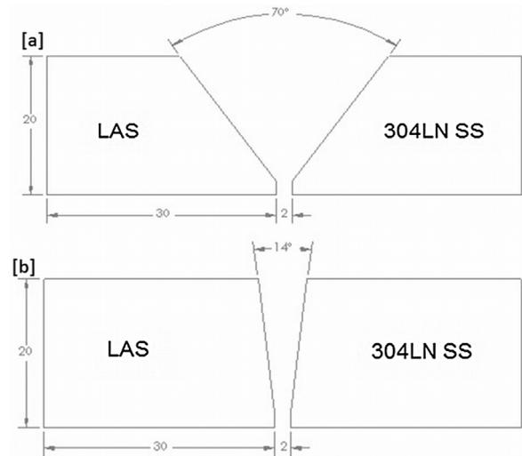
**Fig. 1.** Geometry of welded specimen (a) GTAW and (b) NGW (dimensions are in mm, not to scale).
