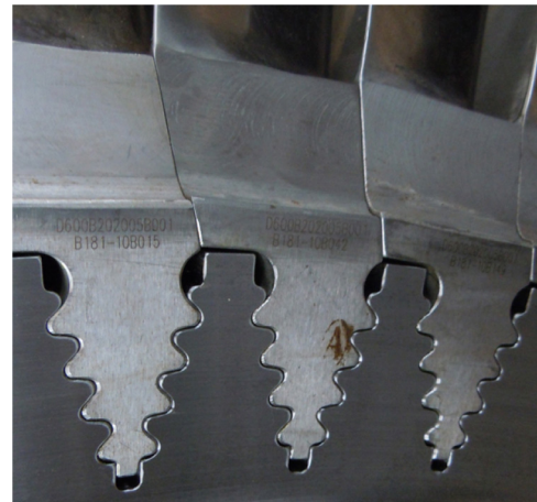
Fig. 2. Fitting between blade roots and slots on rotor disk.
