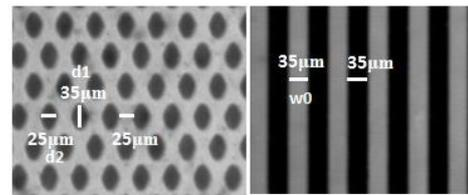
Fig. 1. Photolithography masks of configuration A (left) and B (right).
