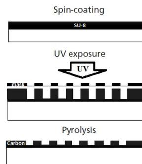
Fig. 2. Schematic illustration of patterns production process: the UV exposure of the 50  $\mu\text{m}$  SU-8 3050 base layer is followed by pyrolysis to obtain carbon structures. The reduction of the pattern thickness is due to the heat treatment occurring during pyrolysis.
