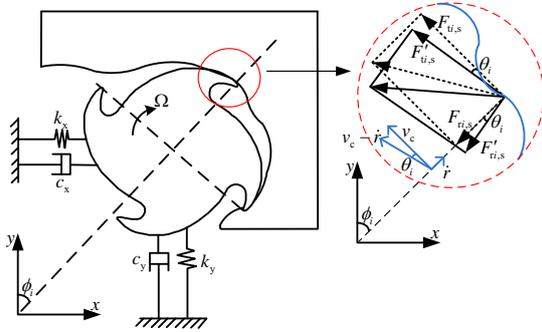
Fig. 1. Process damping due to the velocity effect.
