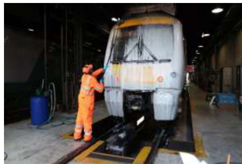
Figure 1: Member of the depot staff performing the cleaning procedure of the train cab front.
