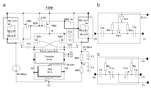
Fig. 2. The schematic of (a) LC-VCO, (b) one branch of 5 bit SCA, and (c) one branch of varactor array.
