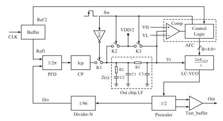
Fig. 1. Block diagram of the proposed PLL.
