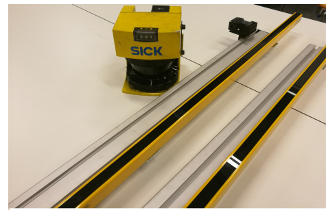
Fig. 2: Examples of safety equipment. The SICK scanner [20] is able to monitor multiple planar zones. The RecR [21] (right) laser curtains consisting of an emitter and receiver is able to monitor a planar region and is used to detect full/partial body (hands) intrusions.
