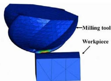
Fig. 1. FE geometry of the ball end milling operation.
