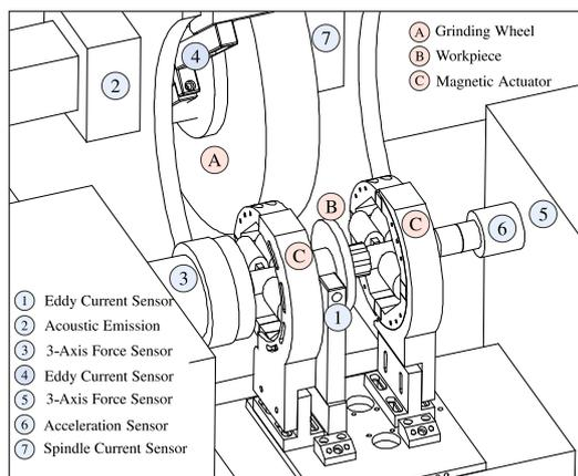
Figure 2: Measurement Setup
