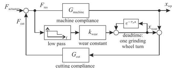
Figure 1: Simplified Grinding Process Model for Wheel-Sided Chatter Vibration in Time Domain by Snoeys & Brown, cf. [1]
