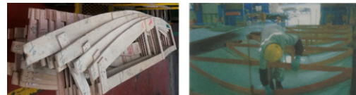
Fig. 1. Evaluation of plates using 2-D template
