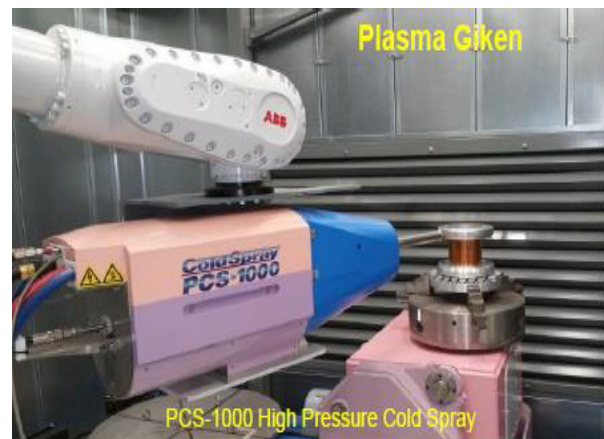
Figure 2: Cold spray with 6 Axis robot and turn-tilt table [7]
