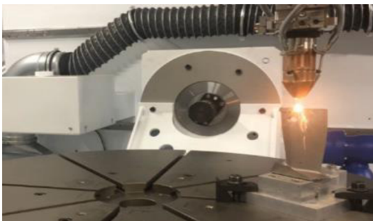
Figure 1: LMD for blade tip repair.
