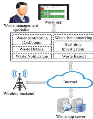
Figure 1 System architecture of real-time waste monitoring
