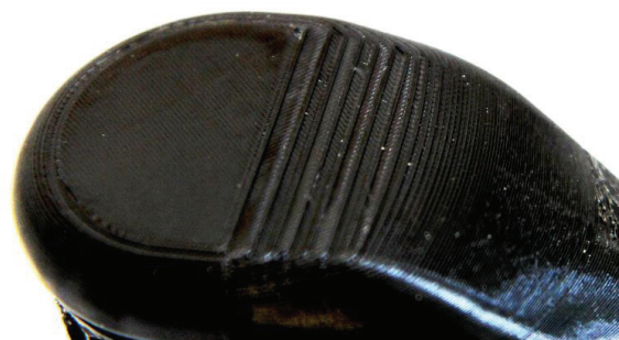
Fig. 2: Stair-step effect on a handle of a walking frame
