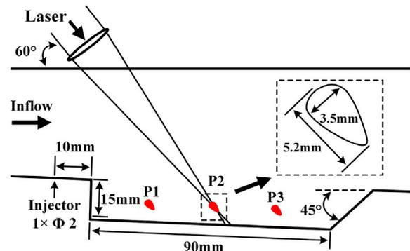
Fig. 2. Schematic of cavity and optics.
