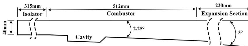
Fig. 1. Schematic of the model scramjet engine and cavity installation.
