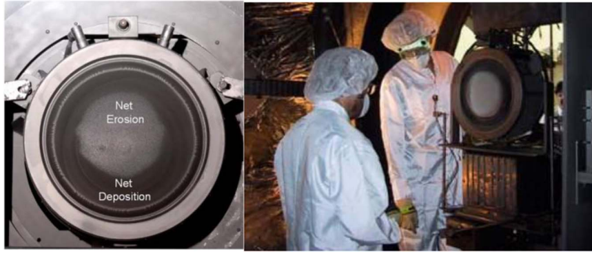
Fig. 1. The net erosion and net deposition areas on the accelerator grids of NEXT LDT (left) [3] and NSTAR ELT (right) [9].
