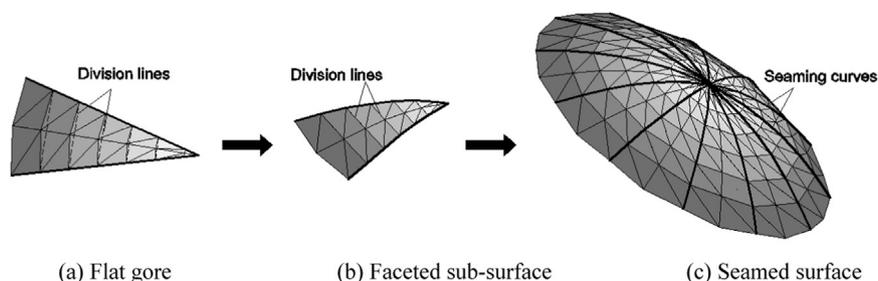
Fig. 2. Modeling the assembly of the initial surface.
