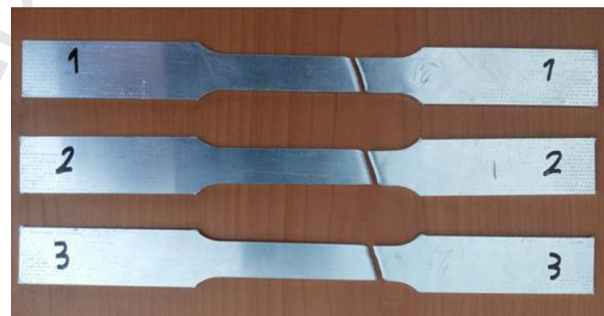
Fig. 2. Tensile test samples.
