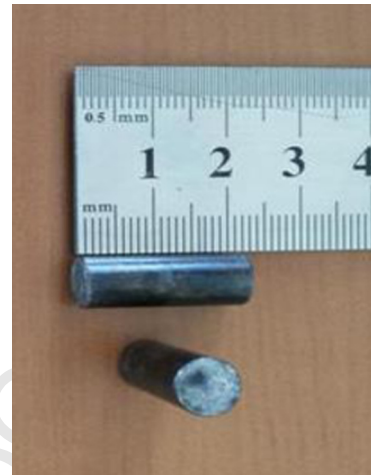
Fig. 1. A view of the projectile used in experimental tests.
