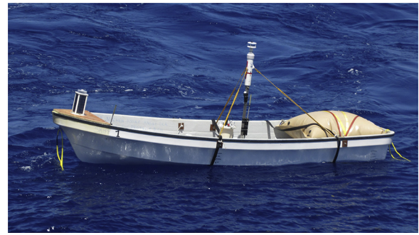
Fig. 2. Photo of a 5.8 m (19-foot) panga skiff loaded with current meter, wind station, GPS iridium beacons, flasher unit, and sandbags to replicate 2 POB loading, as tested during the Leeway field test.
