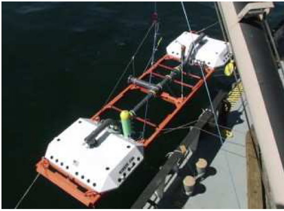
Fig. 1. The scale prototype of the M3 WEC during its deployment offshore the coast of Oregon in September 2014. Photo courtesy of M3 Wave LLC.
