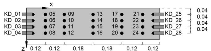
Fig. 1. Distribution of the pressure transmitters in the pit containing the muddy soil (dimensions in metres).
