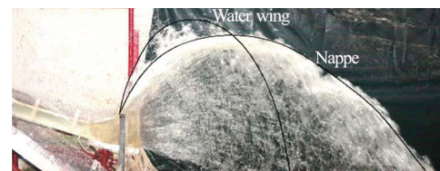
Fig.3 (Color online) Side view of flow through a STED
