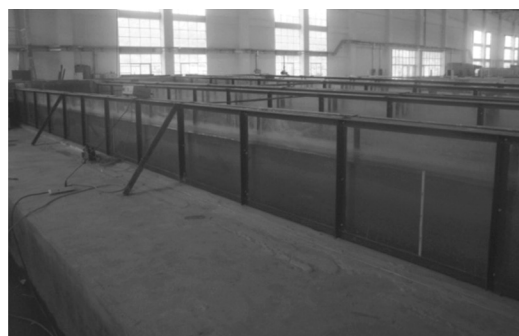
Fig.1 The environmental test channels for measuring the pollution decaying coefficients with water flowing
