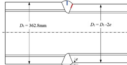
(c) Weld misalignment – unequal diameters ( $D_1 \neq D_2$ )
