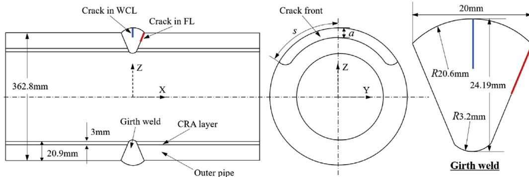
(a) Details of aligned clad pipeline geometry and canoe shape surface crack
