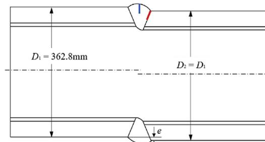
(b) Weld misalignment – equal diameters ( $D_1 = D_2$ )
