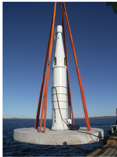
(a) A linear generator before deployment
