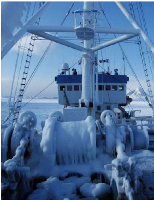
Fig. 1. View of ice accumulation on deck of a marine vessel (Cammaert, 2013).
