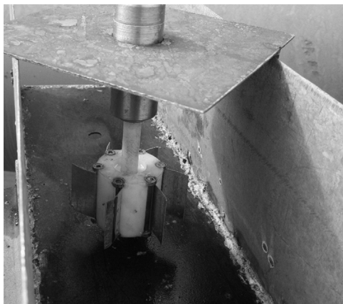
Fig. 2. Turbine position in open channel test rig.
